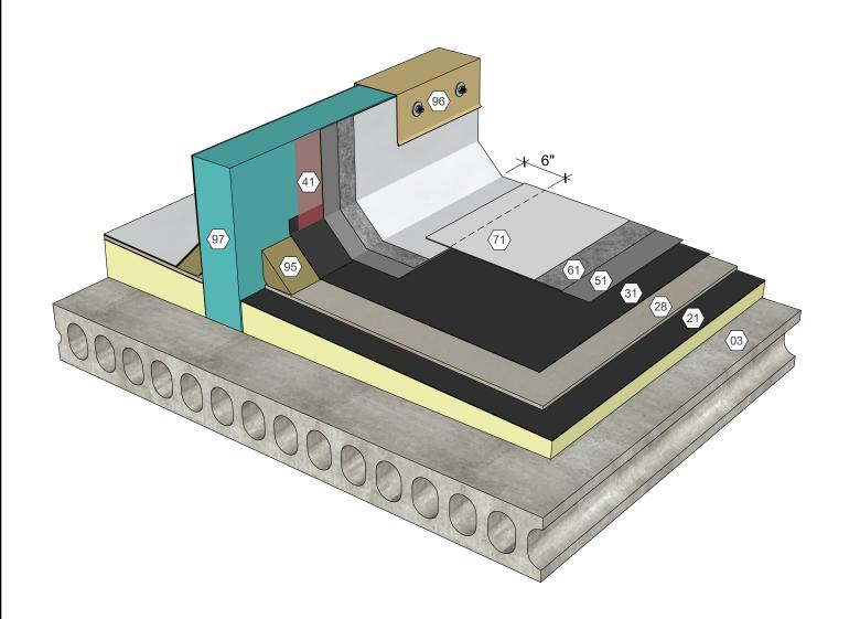
AlphaGuard® MT/MTS Plus Equipment Support Detail, Precast Concrete Deck
